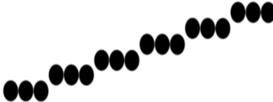
Fig. 2.1: - Stair step effect produced when line is generated as a series of pixel positions.
